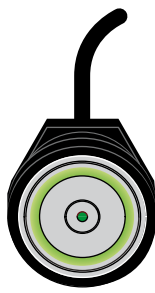
Reader LED turns green (enrolled key)
