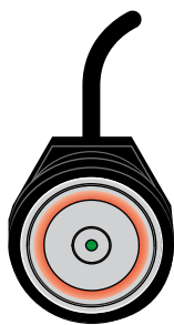
Reader LED turns amber (programming mode)
